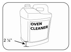
4. Check the degreaser to ensure you have enough to run the AutoClean at the end of the day. If there is less than  $3\frac{1}{2}$ " left, replace the bottle.
