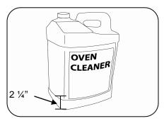
1. Check that the level of degreaser is enough to run the AutoClean. If there is less than 2 ¼" left, replace the bottle.
