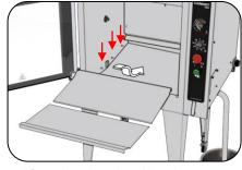
**17.** After cleaning the drip plates, reinstall them into the bottom of the rotisserie by resting the plates on the support pins.
