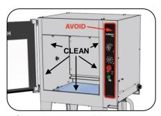
**10.** Clean the interior of the rotisserie: side walls, back wall, bottom pan and exterior of oven around door opening (stainless steel) avoiding the control panel (black).
