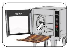
**2.** Remove the drip plates from the bottom of the rotisserie and place in a large sink to be cleaned.
