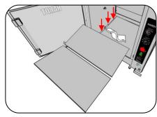
**2.** If applicable, install the drip trays inside the rotisserie by resting them on the support pins.
