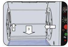
**8.** Lift the left end of the drive assembly and shift to the left to release it. Remove from the rotisserie.
