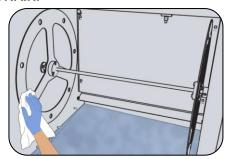
**6.** Clean the drive assembly in the oven and rinse using the water that is in the rotisserie pan.
