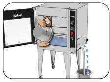
**7.** Pour hot water into the rotisserie pan to clear away any residual grease.
