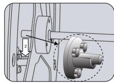
**5.** Then, lower the left end of the drive assembly into its bracket.
