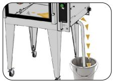
**4.** The grease will flow slowly at first and then increase as the blockage melts.
