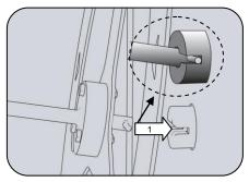
**4.** Insert the right end first by placing the pin on the drive assembly into the groove of the rotator.
