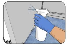
**9.** Spray degreaser on the walls and bottom of the rotisserie's pan; let it set for 10 minutes.
