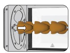
**10.** The triangular end on the left will drop out of the drive plate into your hand. (right end if unloading from the front). Remove the skewer from the rotisserie. Using the green button to advance the drive, continue to unload until all skewers have been removed.
