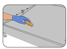
3. Remove all debris, chicken parts, wings, bones, etc. from the bottom of the rotisserie pan and put into the garbage. DO NOT PUSH THE DEBRIS INTO THE DRAIN.
