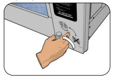
**13.** Open the drain valve to drain the rotisserie then rinse away all degreaser using a soft cloth and clean hot water.
