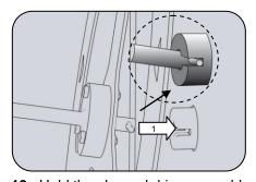
**19.** Hold the cleaned drive assembly with the triangles on the right side. Insert the right end first by placing the pin on the drive into the groove of the rotator.
