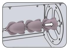
3. Place the V shaped end of the skewer into the triangular socket on the right. Using the green button, advance the drive. Repeat until all skewers are loaded.
