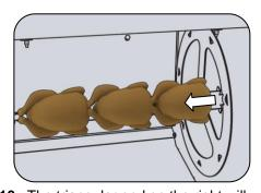
**10.** The triangular end on the right will drop out of the drive plate into your hand. Remove the skewer from the rotisserie. Using the green button to advance the drive, continue to unload until all skewers have been removed.
