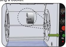
**7.** Using the green button, rotate the drive until the groove on the right side is horizontal.
