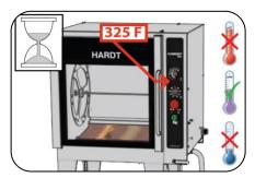
1. Allow the oven to cool until it is comfortable to clean it. If the oven has been turned off and is completely cool, heat up the oven for 10 minutes or to 325 F.
