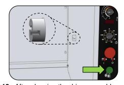
**18.** After cleaning the drive assembly, use the green button to rotate the drive until the groove on the right side is horizontal.
