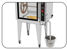
**1.** Ensure that there is a grease reservoir or bucket under the drain.
