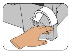
**7.** Ensure that there is no water in the bottom of the rotisserie pan and open the drain valve.
