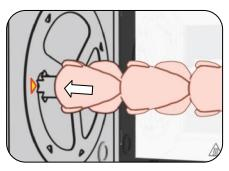
**3.** Place the V shaped end of the skewer into the triangular socket on the left (right side when loading from the front). Using the green button, advance the drive. Repeat until all skewers are loaded.
