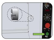
**3.** If applicable, install the drive assembly into the rotisserie. Use the green button to rotate the drive until the groove on the right side is horizontal.
