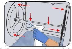
**5.** Spray degreaser on the drive shafts and plates of the drive assembly; let it set for 10 minutes.
