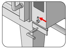
6. After several minutes of preheating (the temperature should read at least 200° F) fill the water pan by opening the water valve.
