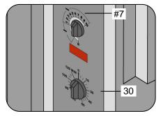
4. Set the thermostat to #7 and the timer to 30 minutes. Pull the red button to start preheating the rotisserie. The burner will ignite after about 1 minute and the rotisserie will start to preheat.
