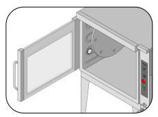
1. Ensure that the rotisserie has been properly preheated at #7 for 30 minutes. When the rotisserie is preheated and alarm will sound. Open the door. The burner will switch off and the drive will stop.
