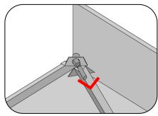
2. If using the horizontal skewer rack and skewering table; take a skewer and place the hex end into the hole at the back left corner of the prep table. The skewer should be positioned with the "V" pointing down.
