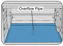
7. Fill water to the top of the overflow pipe then close the water valve. CAUTION: Do not walk away from the rotisserie while filling the pan.
