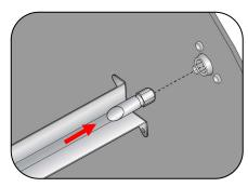
3. Place the hexagonal end in the socket on the right. Ensure the skewer is locked in place and that the breast is facing out. Press the green manual advance switch to rotate the drive to load the next skewer.
