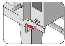
8. Drain the water pan by opening the drain valve. Rinse the water pan.
