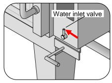
12. Open the water inlet valve to raise the water to the level indicated in the following step.
