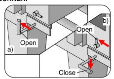
6. Drain the water pan (a) and then fill it with clean water (b). Rinse the cavity to remove any degreaser.
