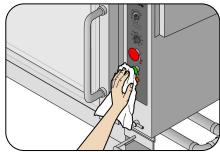
11. Clean the exterior of the rotisserie especially the top front cover, the control panel and the legs. **DON'T USE A STRONG CLEANER ON THE CONTROL PANEL.**
