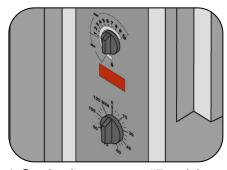
4. Set the thermostat to #7 and the timer according to the chart to the right.
