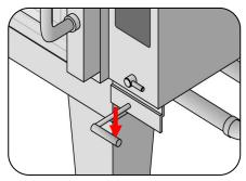
3. Ensure that there is no water in the water pan and close the drain valve. Always drain all water from the water pan prior to preheating.
