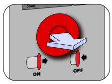
3. Verify that the gas supply to the rotisserie and the main gas valve are both open. Try to start the unit again by pulling out the red main ON/OFF switch. If the unit goes into SAFETY LOCK OUT again, push in the red main ON/OFF switch.
