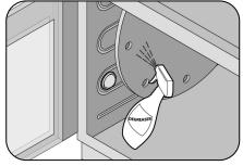
3. Spray degreaser on the drive plate, support plate, center shaft and side walls. Let set for 10 minutes. **DO NOT SPRAY DEGREASER ON THE BURNER.**
