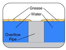
13. Raise the water until the grease is skimmed off down the drain as shown above.
