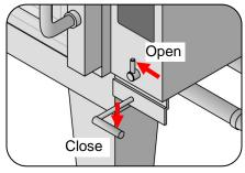
4. Close the drain valve and open the water valve. Fill the water pan with clean water.
