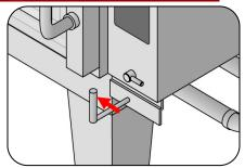
1. Open the drain valve to drain the greasy water from the water pan.
