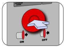
2. Push in the red main ON/OFF switch to switch the rotisserie OFF.
