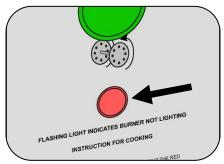
1. If the red main ON/OFF switch is pulled and the igniter glows several times but there is no flame the unit has gone into "SAFETY LOCK OUT". The red light below the green button will flash.
