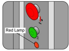
5. If a safety lock-out occurs, the red lamp on the control panel will blink. Follow the safety lock-out instructions on the sheet provided.
